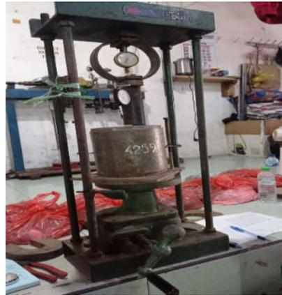
Gambar 8 Tes uji nilai CBR laboratorium
