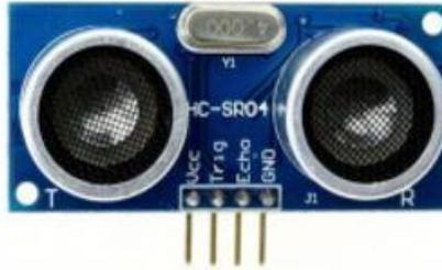
Gambar 4. Sensor Ultrasonik HCSR-04
