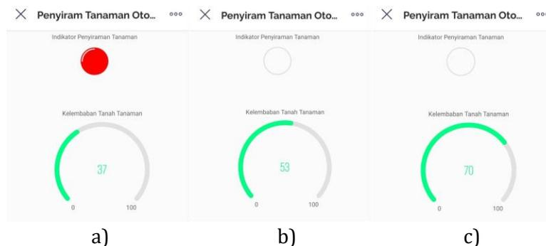
**Gambar 3.** Tampilan Blynk App Monitoring Tanaman. (a) Tampilan monitoring kelembapan tanah kering, (b) Tampilan monitoring kelembapan tanah lembap, (c) Tampilan monitoring tanah basah
