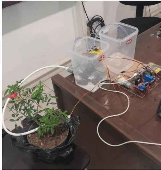
Gambar 4. Alat Monitoring Tanaman Otomatis Berbasis IoT
