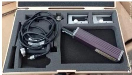
**Gambar 4.** Mitutoyo SJ 310 Surface roughness Tester
