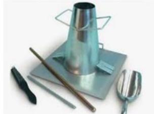
Gambar 4. Slump Flow (kerucut abrams)
