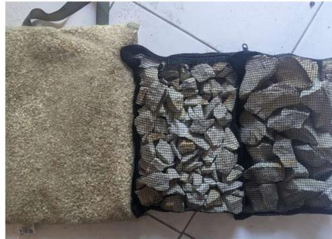
Gambar 1. Media filter zeolit
