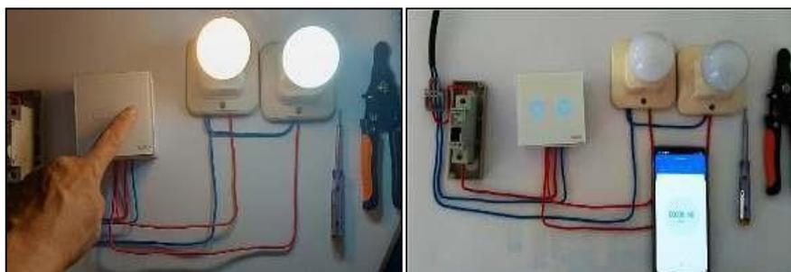
Gambar 7. Rangkaian uji coba sakelar pintar Bardi *smart wall switch*
