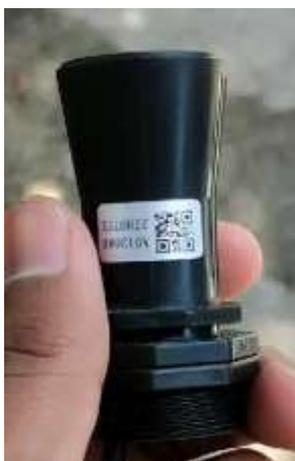
Gambar 5. Sensor Level ultrasonic
