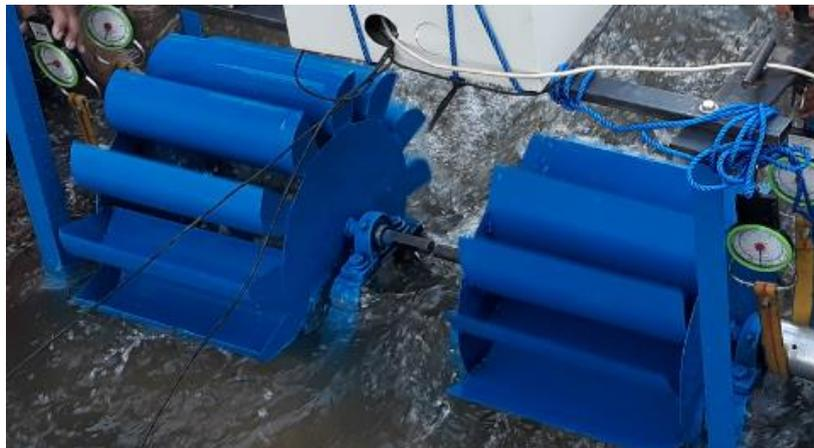
Figure 3. Undershot type waterwheel
