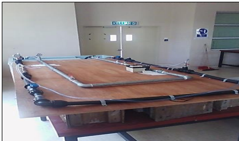
Fig. 3. Test rig for MDPE pipeline leak detection
