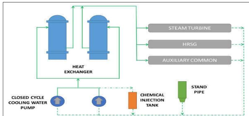
Figure 2. Steam Turbine Closed Cooling System
