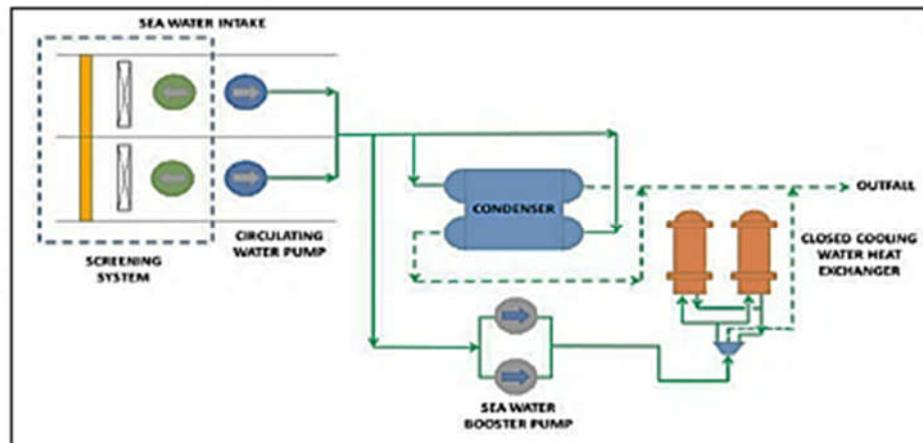
Figure 3. Steam Turbine Pltgu Grati Open Cooling System
