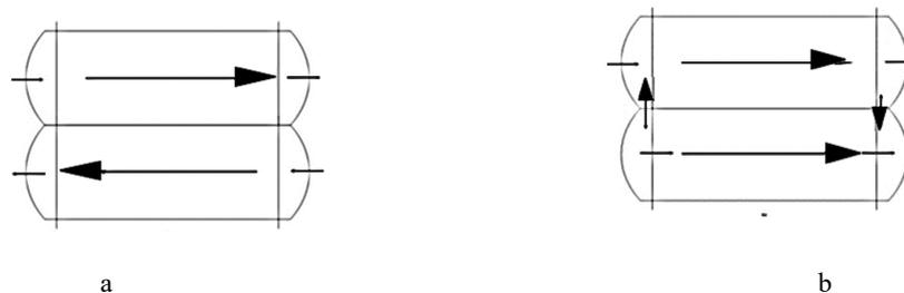
Figure 4. (a) Normal condenser flow direction, (b) direction of condenser flow during backwash
