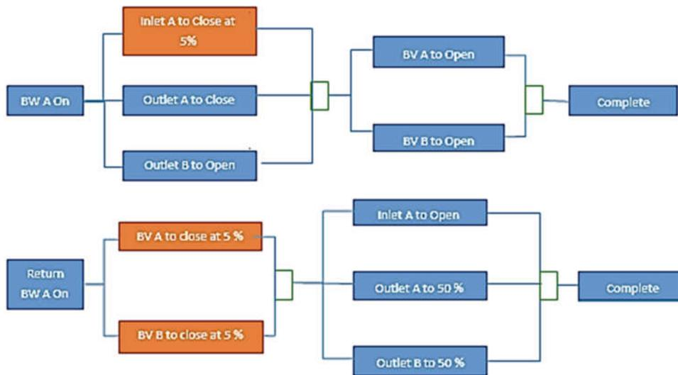
Figure 7. The B-side condenser backwash process is the opposite of the A-side condenser backwash.
