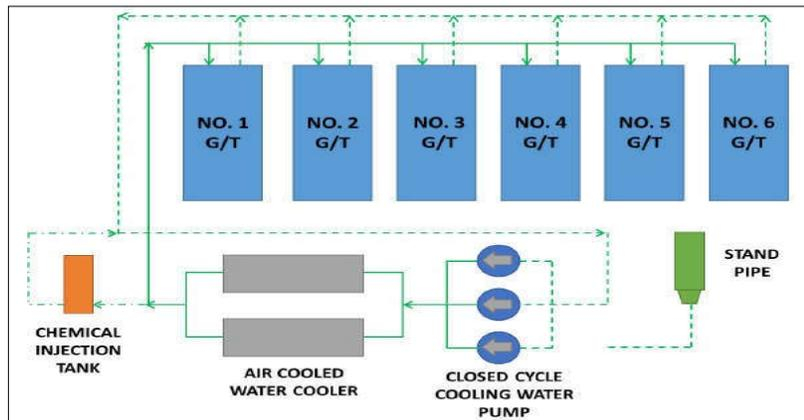
Figure 1. Gas Turbine Closed Cooling System
