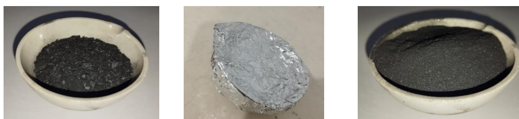
Figure 1. (a) Sappan wood charcoal, (b) Activator solution mixing process and (c) Sappan wood activated charcoal.
