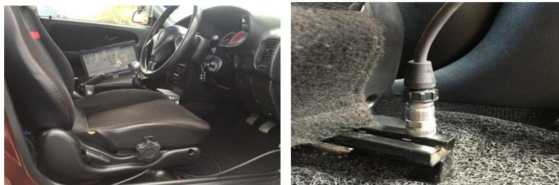
Fig. 4. Accelerometer attached on the car seat.
