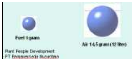
Gambar 2. Excess Air Ratio Sumber : Komatsu Diesel Engine
