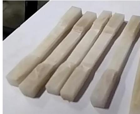
Gambar 8. Hasil spesimen ASTM D3039
