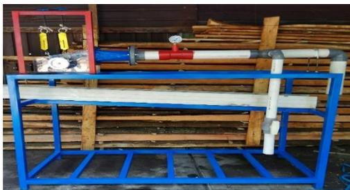
Gambar 4 Alat uji turbin crossflow
