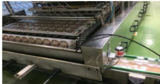
Gambar 1. Mesin *filling cup sealer*
